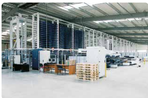
Automated warehouse for sheet steel and parts
