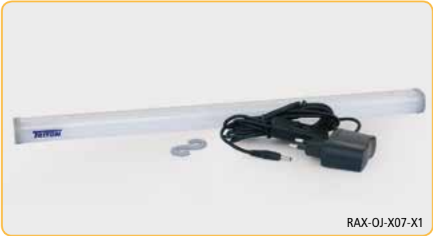
RAX-OJ-X07-X1 LED-diode lighting unit with magnet 1/2U with possibility of fixing on the vertical 19" rails, external power supply 230 V, 315 lm.
