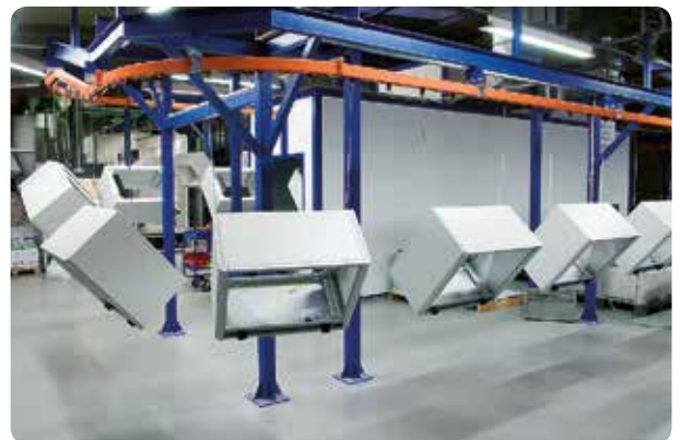
Paintshop - powder coating line
